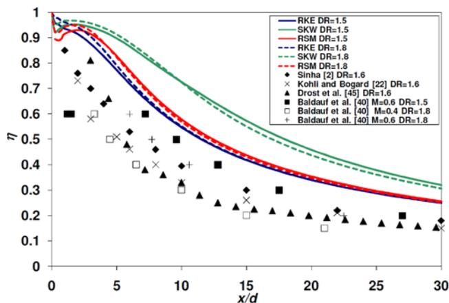
Fig. 6 Predictions of centerline  $\eta$  distributions using various turbulence models for  $M = 0.5$
