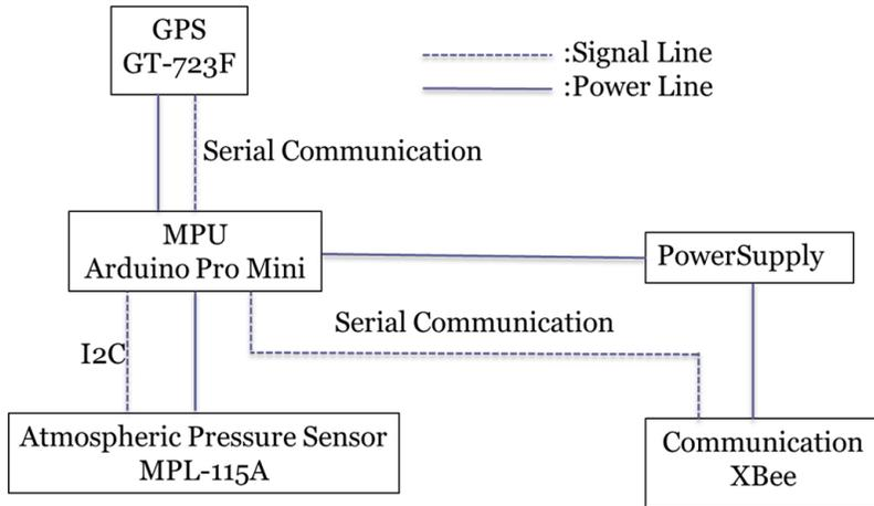
Figure 8. Block diagram of proposed avionics system.
