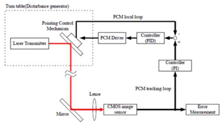
Figure 11. Block diagram for on-board system.
