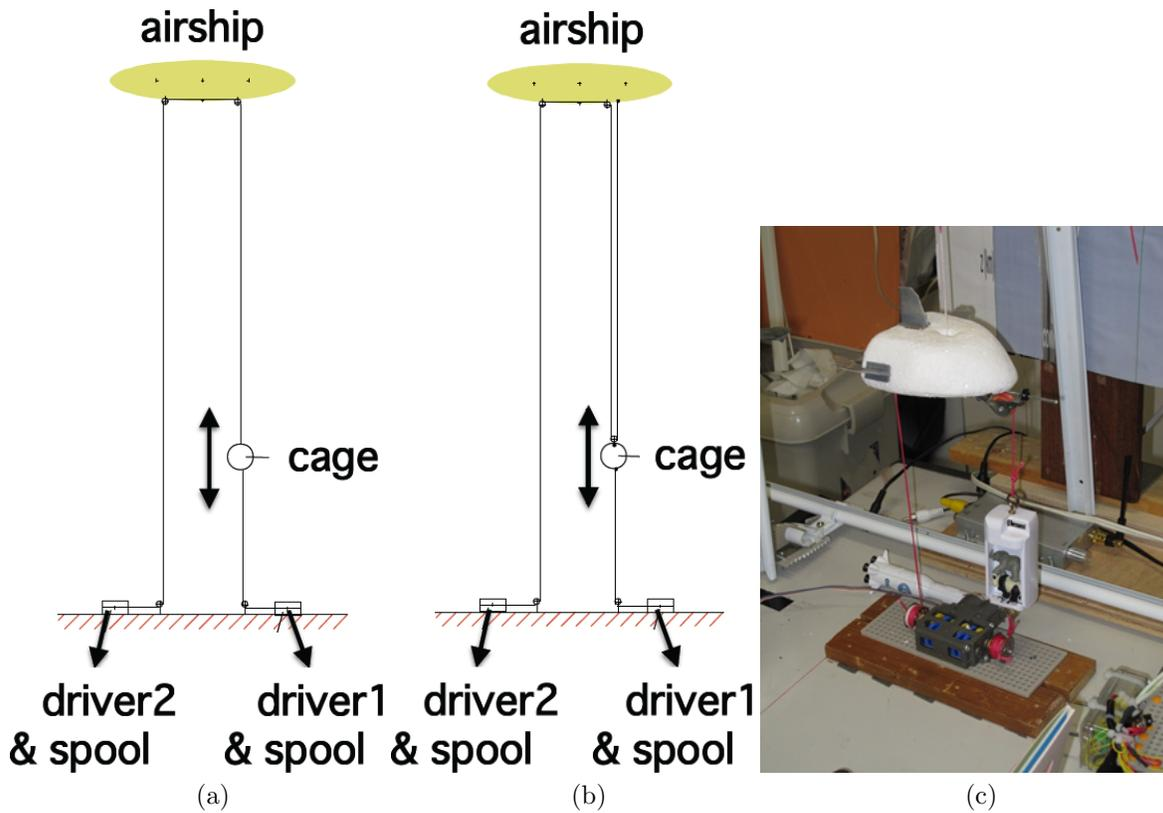
Figure 7. Two types of elevator systems. (c) is a trial-made model of type (a).
