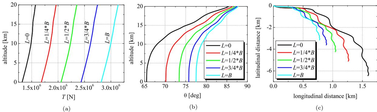
Figure 4. Effects by  $L$ -variations on the tether cable. (a) Tether cable tension  $T$  versus altitudes. (b) Tether cable elevation angle  $\theta$  versus altitudes. (c) Tether cable silhouettes projected onto the ground, namely  $x$ - $y$  plane; ground mooring point as their origin.
