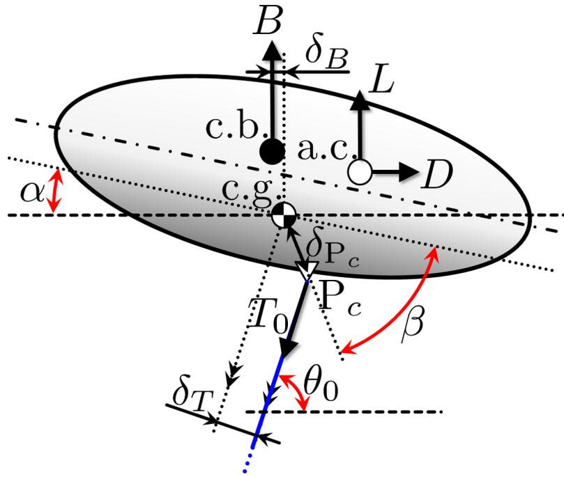
Figure 5. Diagram for analysis on pitching stability; aerodynamic center “a.c.”, center of buoyancy “b.c.”, center of gravity “c.g.”, connecting point of hull to tether rope top end “ $P_c$ ”. Blue colored line shows tether cable.
