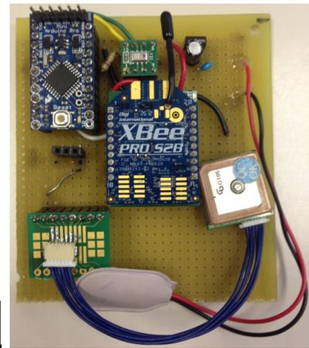
Figure 9. Developed avionics equipment.
