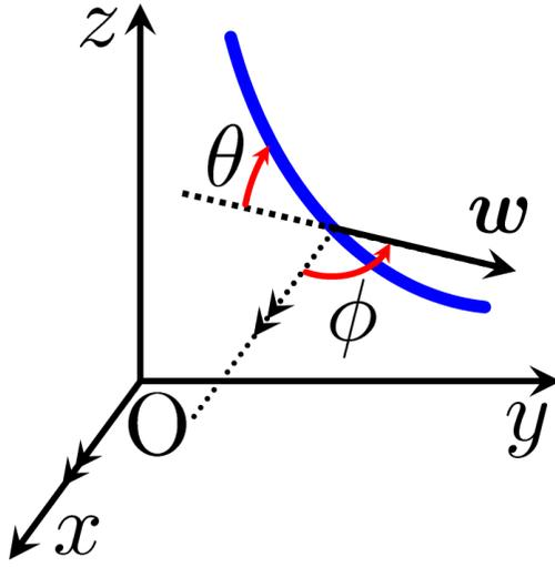
**Figure 1. Coordinate system for behavioral analysis of the captive high-altitude platform system comprised with an LTA vehicle and a tether cable. Blue colored curve line symbolizes the tether cable.**
