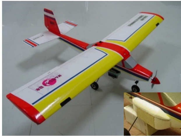
Figure 1. Exterior of utilized sUAV as Prairie. The bottom right is the enlarged figure around the camera mount.
